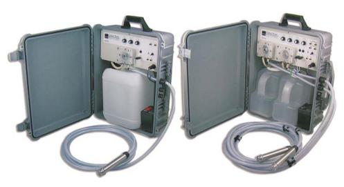
The WS700 single bottle sampler allows you to take a time or flow (with optional flow monitor) weighted composite sample or a discrete (grab) sample.
